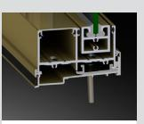
Bottom rail is recessed fully into sill to achieve a clean sight line and minimal appearance
